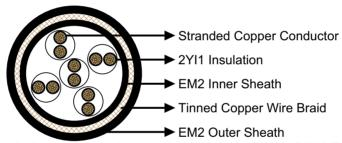
**Conductors:** Flexible stranded copper conductor, class 5 according to DIN VDE 0295. **Insulation:** PE type 2YI1.
